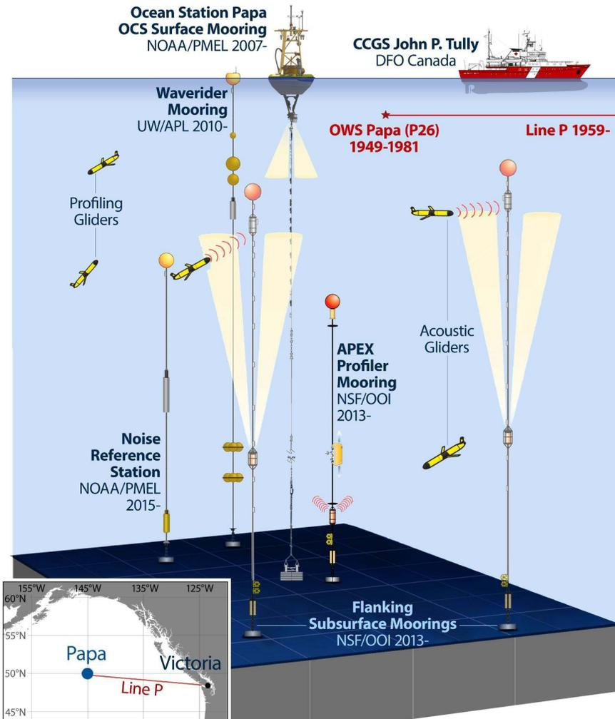
**Figure 1.** Illustration of the operational components of Ocean Station Papa and their respective names and locations. Credit: Sarah Battle, NOAA/PMEL graphic adapted from original by the Ocean Observatories Initiative.
