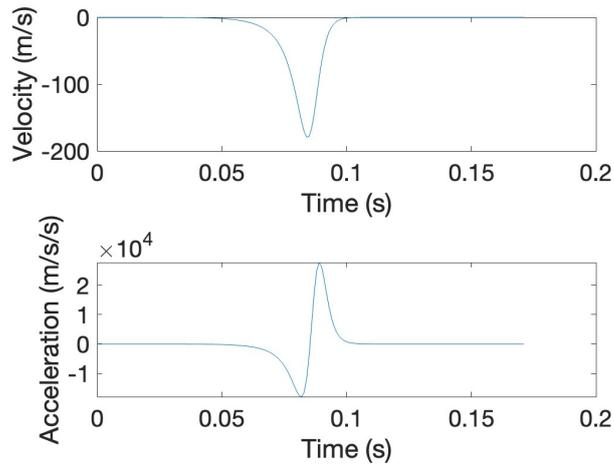
Figure 8: Velocity - time and Acceleration - time graphs: Van der Pol equation:  $\ddot{x} + \mu(x^2 - 1)\dot{x} + x = 0$ ;  $x(0) = x_0$ ,  $\dot{x}(0) = \dot{x}_0$ ;  $\mu = 160$ ,  $\Delta t = 0.001$  seconds; showing peak velocity and peak acceleration and asymptotic curves
