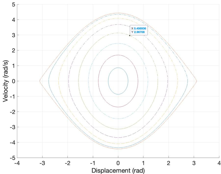
Figure 15: Velocity - displacement graph: Pendulum equation:  $\ddot{\theta} + \frac{g}{l} \sin(\theta) = 0$ ;  $g = 9.81 (m/s^2)$ ; length of pendulum:  $l = 2 (m)$ ; initial  $\theta = \pi/8, 2\pi/8, 3\pi/8, 4\pi/8, 5\pi/8, 6\pi/8, 7\pi/8, 7.9\pi/8 \approx \pi$  (rad) for inner ring, initial  $\theta = \pi/8$ , outer ring, initial  $\theta \approx \pi$ ;  $\Delta t = 0.01$  seconds
