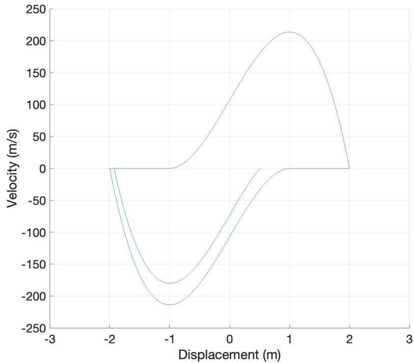
Figure 3: Velocity - displacement graph: Van der Pol equation:  $\ddot{x} + \mu(x^2 - 1)\dot{x} + x = 0$ ;  $x(0) = x_0, \dot{x}(0) = \dot{x}_0$ ;  $\mu = 160$ ; for initial conditions:  $(0.5, 0.0)$ ;  $\Delta t = 0.001$  seconds
