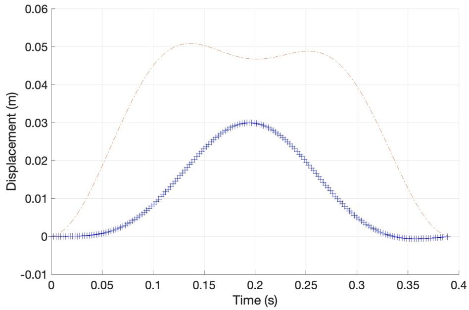
Figure 20: Graph of displacement vs time: 2-dof system;  $x(0) = 0$ ,  $\dot{x}(0) = 0$ ,  $\Delta t = 2.3416e - 06(s)$ ; 2-dof:  $m_{11} = 100, m_{12} = m_{21} = 0, m_{22} = 25; b_{11} = b_{12} = b_{21} = b_{22} = 0; k_{11} = 54000, k_{12} = k_{21} = -18000, k_{22} = 18000; f_1 = 0, f_2 = 400$
