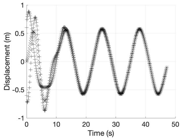
Figure 14: Displacement - time graph: Duffing equation:  $\ddot{x} + \delta\dot{x} + \alpha x + \beta x^3 = \gamma \cos(\omega t)$ ;  $x(0) = x_0, \dot{x}(0) = \dot{x}_0$ . Initial conditions:  $(0, 0), (-6, -6), (6, 6)$ , and constants,  $\delta = 0.4, \alpha = 1, \beta = 0.5, \gamma = 0.5, \omega = 0.5$ ; steady-state conditions reached after 1 cycle
