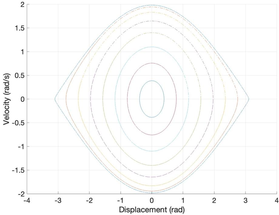
Figure 16: Velocity - displacement graph: Pendulum equation:  $\ddot{\theta} + \frac{g}{l}\sin(\theta) = 0$ ;  $g = 9.81 (m/s^2)$ ; length of pendulum:  $l = 10 (m)$ ; initial  $\theta = \pi/8, 2\pi/8, 3\pi/8, 4\pi/8, 5\pi/8, 6\pi/8, 7\pi/8, 7.9\pi/8 \approx \pi$  (rad) for inner ring, initial  $\theta = \pi/8$ , outer ring, initial  $\theta \approx \pi$ ;  $\Delta t = 0.01$  seconds
