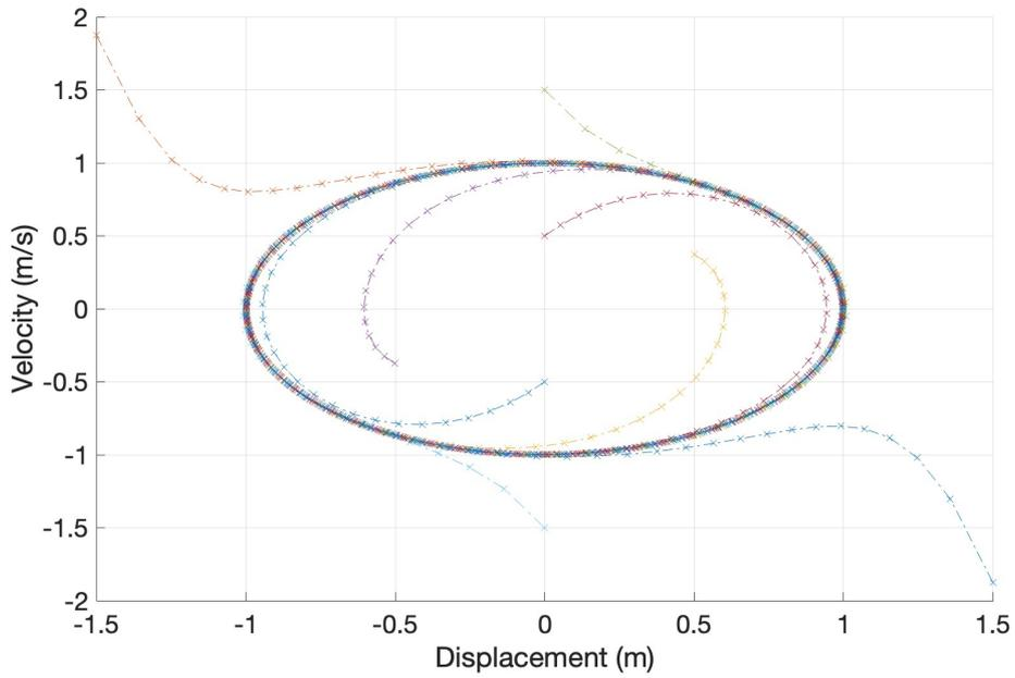
Figure 18: Graph of velocity vs displacement: System- $x_1$ ; initial conditions:  $(1.5,0), (-1.5,0), (0.5,0), (-0.5,0), (0,1.5), (0,-1.5), (0,0.5), (0,-0.5)$ ;  $\Delta t = 0.1, 0.01, 0.001, 0.0001$  seconds, gave same limit cycles.
