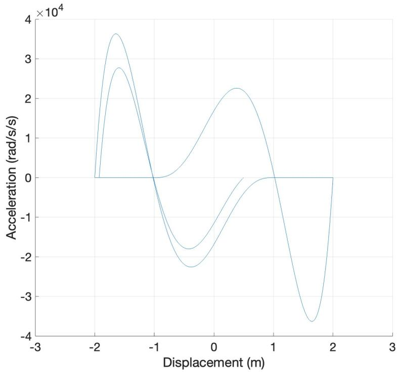
Figure 4: Acceleration - displacement graph: Van der Pol equation:  $\ddot{x} + \mu(x^2 - 1)\dot{x} + x = 0$ ;  $x(0) = x_0, \dot{x}(0) = \dot{x}_0$ ;  $\mu = 160$ ; for initial conditions:  $(0.5, 0.0)$ ;  $\Delta t = 0.001$  seconds
