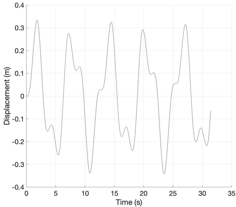
Figure 23: Graph of displacement vs time: 200-dof system;  $\Delta t_0 = 1e - 02(s)$ ; with adaptive time stepping scheme used,  $281.5945e - 6 \leq \Delta t_n \leq 1e - 3(s)$ , CPU time, 965.138(s); fixed  $\Delta t_0 = 1e - 3(s)$ , CPU time, 258.764(s)duration of simulation,  $10\pi(s)$
