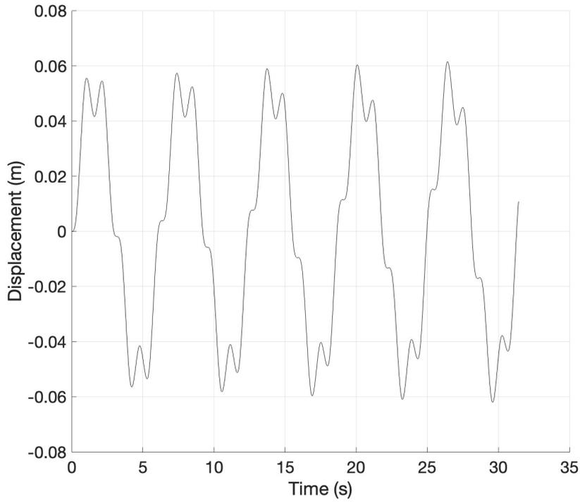
Figure 22: Graph of displacement vs time: 100-dof system;  $\Delta t_0 = 1e - 02(s)$ ; with adaptive time stepping scheme used,  $281.5945e - 6 \leq \Delta t_n \leq 1e - 3(s)$ , CPU time, 254.616(s); fixed  $\Delta t_0 = 1e - 3(s)$ , CPU time, 69.094(s), duration of simulation,  $10\pi(s)$
