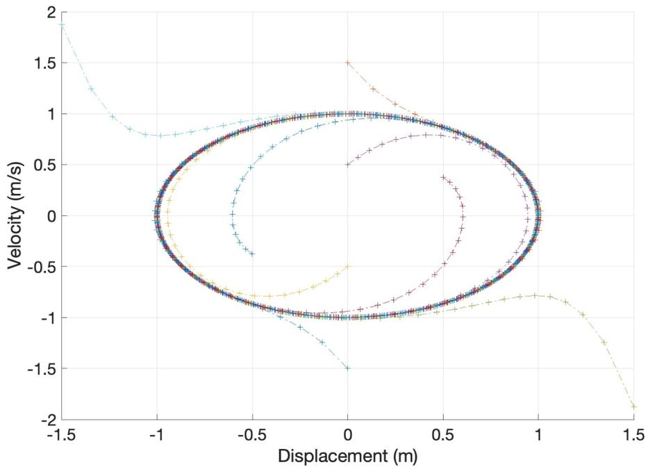
Figure 19: Graph of velocity vs displacement: System- $x_2$ ; initial conditions:  $(1.5,0), (-1.5,0), (0.5,0), (-0.5,0), (0,1.5), (0,-1.5), (0,0.5), (0,-0.5)$ ;  $\Delta t = 0.1, 0.01, 0.001, 0.0001$  seconds, gave same limit cycles.
