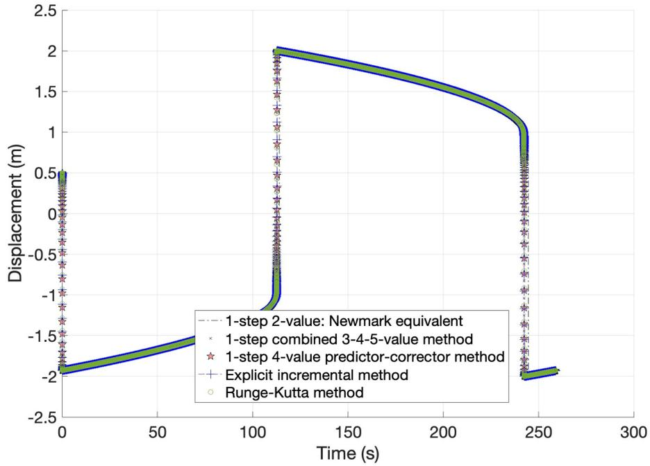
Figure 12: Displacement - time graph: Van der Pol equation:  $\ddot{x} + \mu(x^2 - 1)\dot{x} + x = 0; x(0) = x_0, \dot{x}(0) = \dot{x}_0; \mu = 160$ ; initial conditions:  $(0.5, 0.0)$ ;  $\Delta t = 0.001$  seconds; plotted during profiling functions
