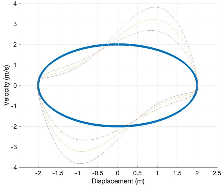
Figure 10: Velocity - displacement graph: Van der Pol equation:  $\ddot{x} + \mu(x^2 - 1)\dot{x} + x = 0; x(0) = x_0, \dot{x}(0) = \dot{x}_0;$
