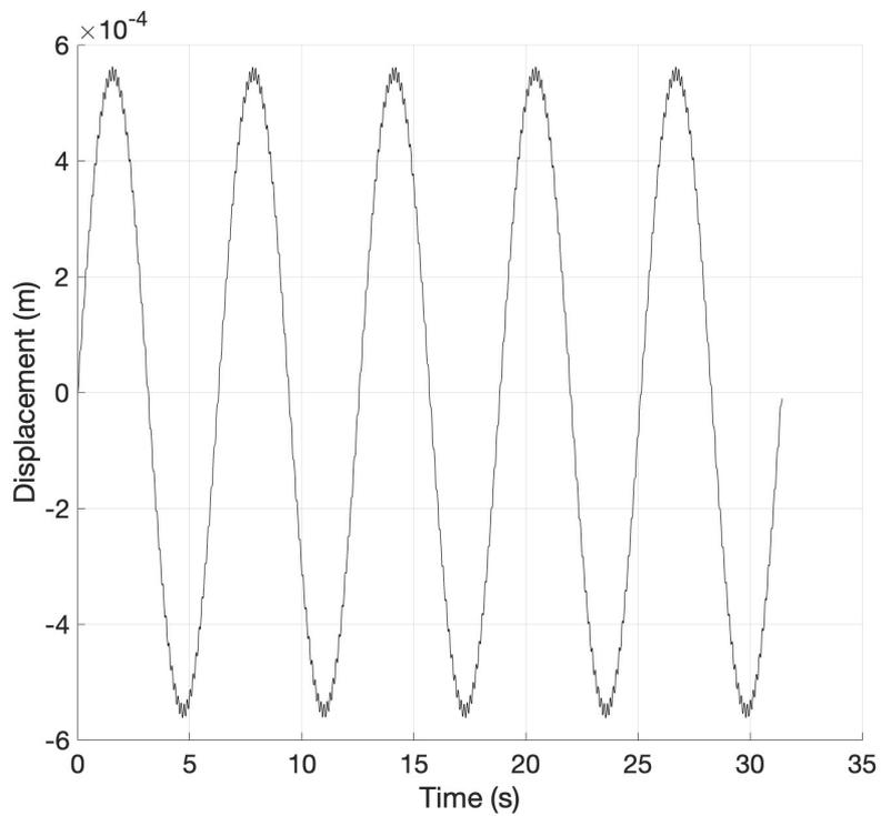
Figure 21: Graph of displacement vs time: 10-dof system; fixed  $\Delta t_0 = 1e - 03(s)$ ; CPU time, 2.197(s), duration of simulation,  $10\pi(s)$
