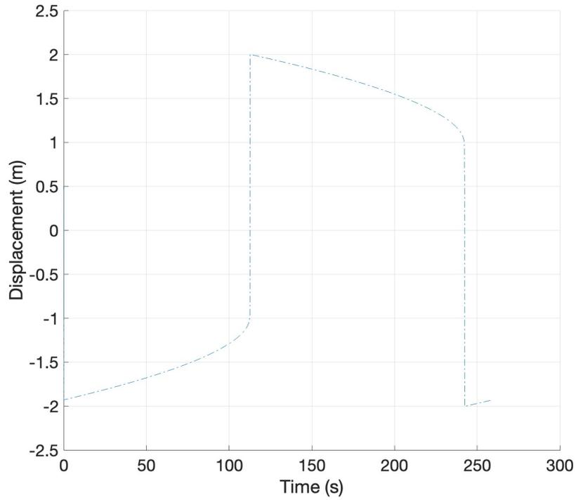
Figure 2: Displacement - time graph: Van der Pol equation:  $\ddot{x} + \mu(x^2 - 1)\dot{x} + x = 0$ ;  $x(0) = x_0, \dot{x}(0) = \dot{x}_0$ ;  $\mu = 160$ ; for initial conditions:  $(0.5, 0.0)$ ;  $\Delta t = 0.001$  seconds
