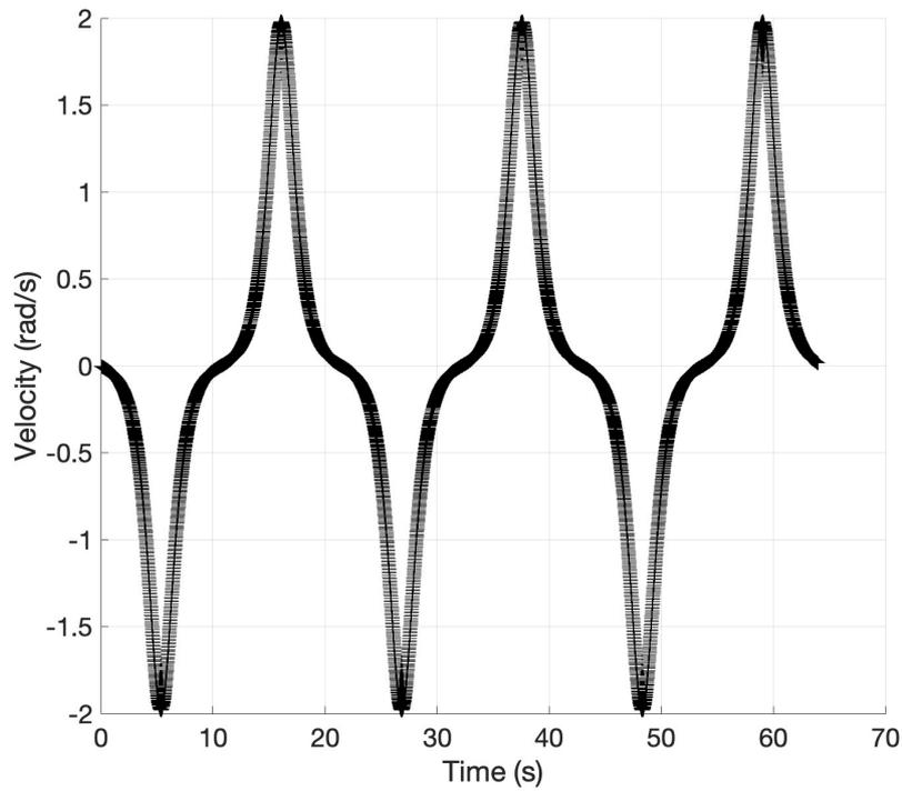
Figure 17: Velocity - time graph: Pendulum equation:  $\ddot{\theta} + \frac{g}{l}\sin(\theta) = 0$ ;  $g = 9.81 (m/s^2)$ ; length of pendulum:  $l = 10 (m)$ ; initial  $\theta = 7.9\pi/8 \approx \pi$  (rad);  $\Delta t = 0.01$  seconds
