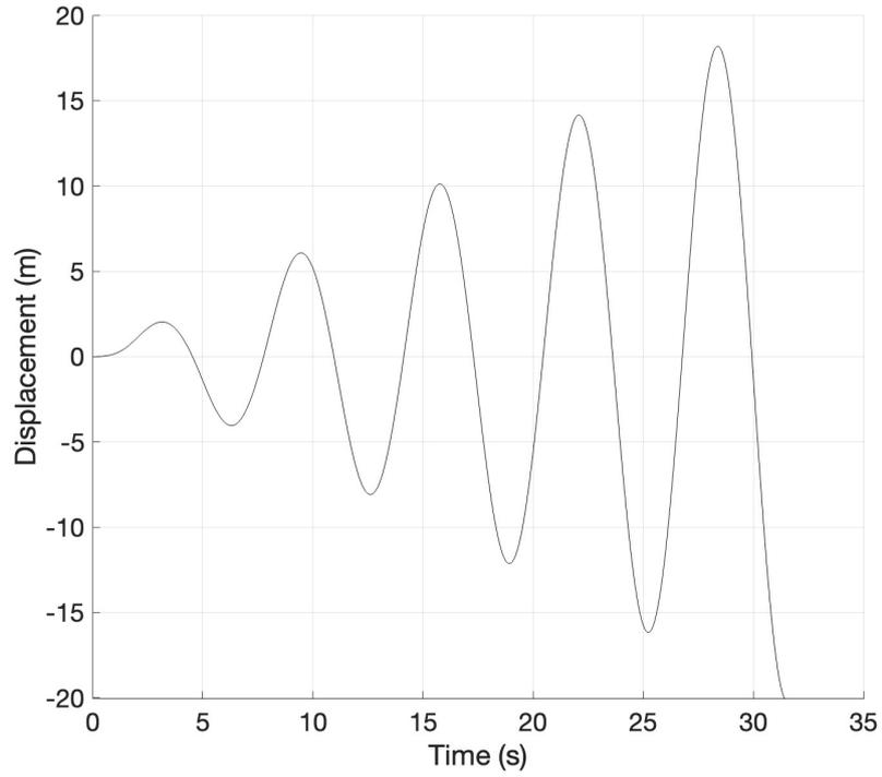
Figure 24: Graph of displacement vs time: 500-dof system;  $\Delta t_0 = 1e - 02(s)$ ; with adaptive time stepping scheme used,  $281.5945e - 6 \leq \Delta t_n \leq 1e - 3(s)$ , CPU time, 5380.668(s), fixed  $\Delta t_0 = 1e - 03(s)$ , CPU time, 1478.304(s), duration of simulation,  $10\pi(s)$
