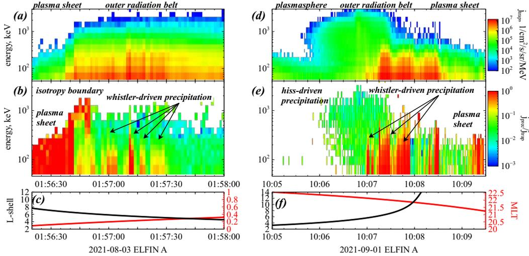
**Figure 1.** Two examples of ELFIN observations with strong precipitation of energetic electrons in the nightside MLT sector showing locally trapped electron fluxes (a,d), precipitating-to-trapped flux ratio (b,e), and ELFIN’s MLT,  $L$ -shell coordinates from (Tsyganenko, 1989) model (c,f).
