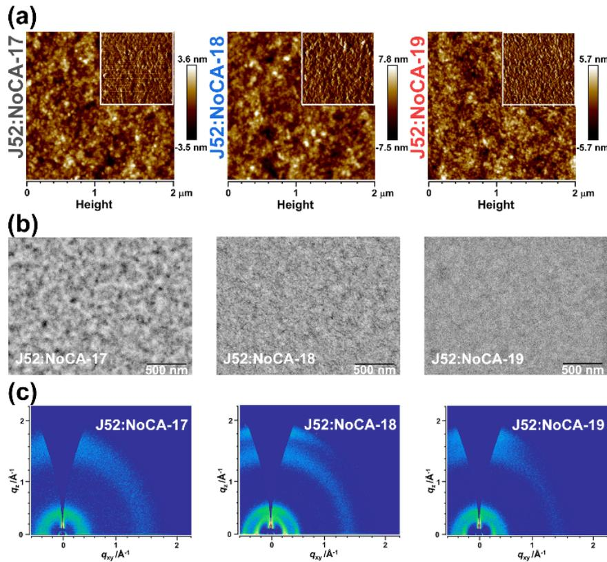
**Figure 4** (a) Tapping-mode AFM height images ( $2\ \mu\text{m} \times 2\ \mu\text{m}$ ) (insets are phase images of  $1\ \mu\text{m} \times 1\ \mu\text{m}$  size), (b) TEM images, and (c) 2D-GIWAXS patterns of J52:NoCA-17, J52:NoCA-18, and J52:NoCA-19 blend films.
