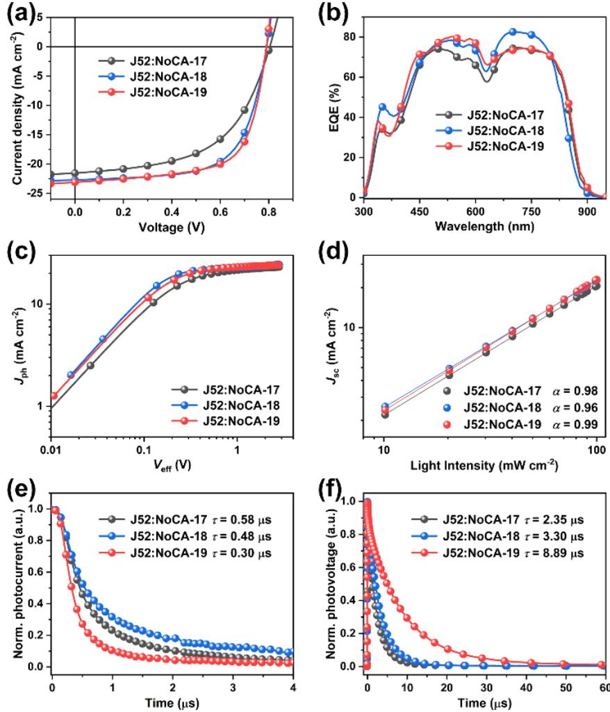
**Figure 3** (a)  $J$ - $V$  characteristics, (b) EQE responses, (c)  $J_{\text{ph}}-V_{\text{eff}}$ , (d)  $J_{\text{sc}}-P_{\text{light}}$ , (e) TPC, and (f) TPV measurements of the optimized OSCs based on J52:NoCA-17, J52:NoCA-18, and J52:NoCA-19.
