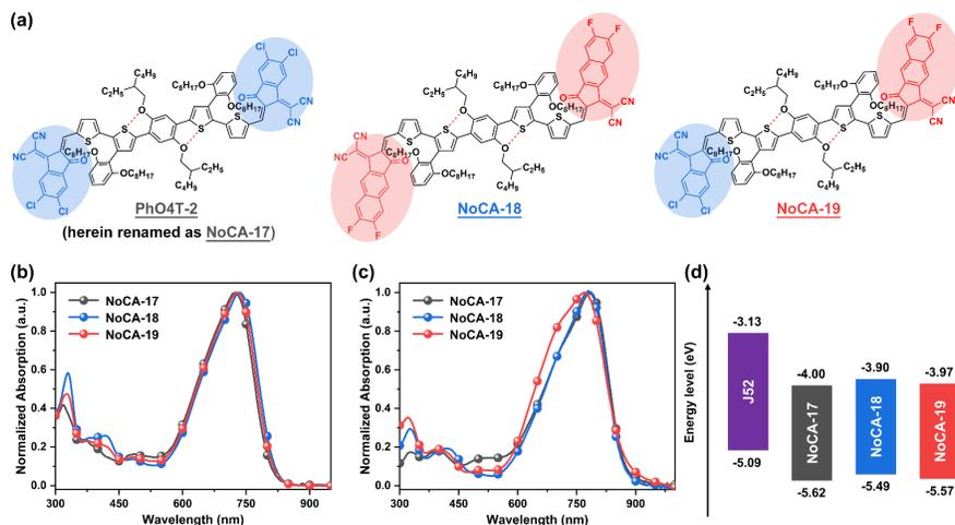
**Figure 1** (a) Chemical structures, normalized dilute solution (b) and thin film (c) optical absorption spectra of the three NRFEAs. (d) Energy level diagram of donor and acceptor materials in this work.
