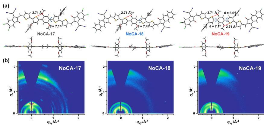
**Figure 2** (a) Optimized geometries (top: top view; bottom: side view) of the three NFREAs. (b) 2D-GIWAXS patterns of neat NoCA-17, NoCA-18, and NoCA-19 films.
