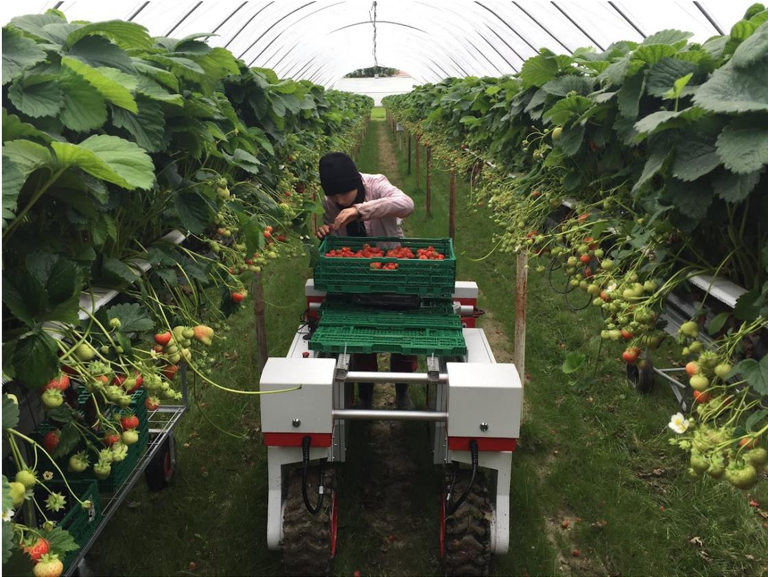
Figure 7: The Thorvald robot used for a fruit transportation task.
