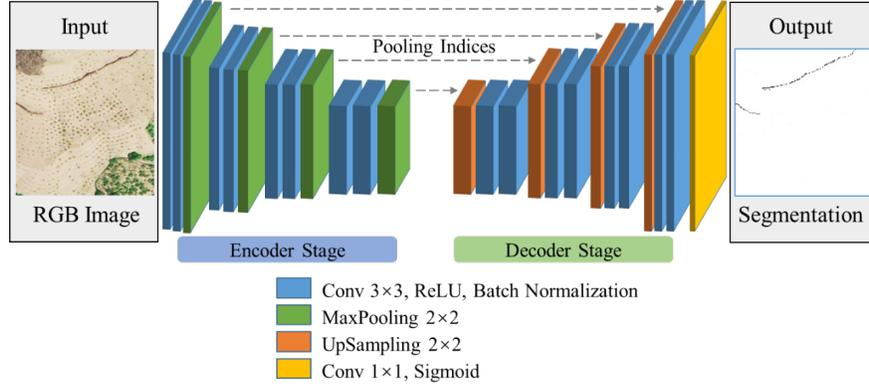
Figure 3. Network structure diagram of the SegNet model.
