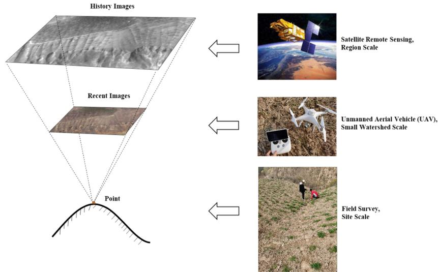
Figure 2. Three spatial scale ephemeral gully monitoring methods.
