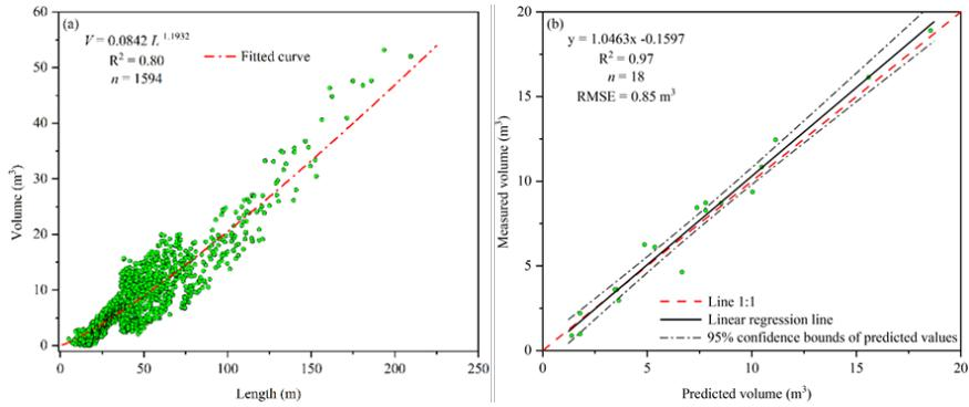
Figure 6. Establishment and verification of the  $V-L$  model. (a) Power relationshi between ephemeral gully volume ( $V$ ) and ephemeral gully length ( $L$ ). (b) Comparison of predicted ephemeral gully volume with measured ephemeral gully volume.
