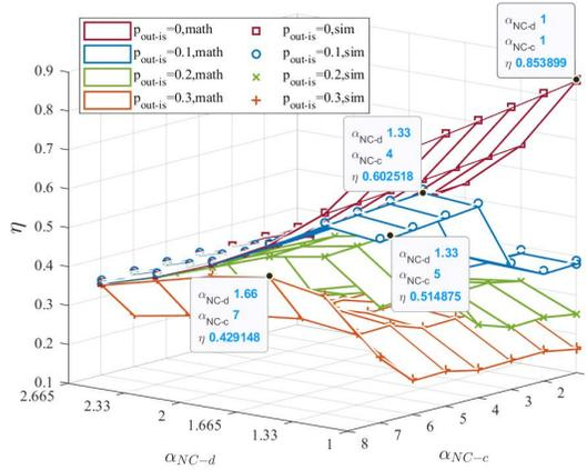
**FIGURE 6** Resource efficiency of the DENC under different outage probabilities of ISLs and coding coefficients. As the coding coefficient increases, math, the resource efficiency rises first and then drops.
