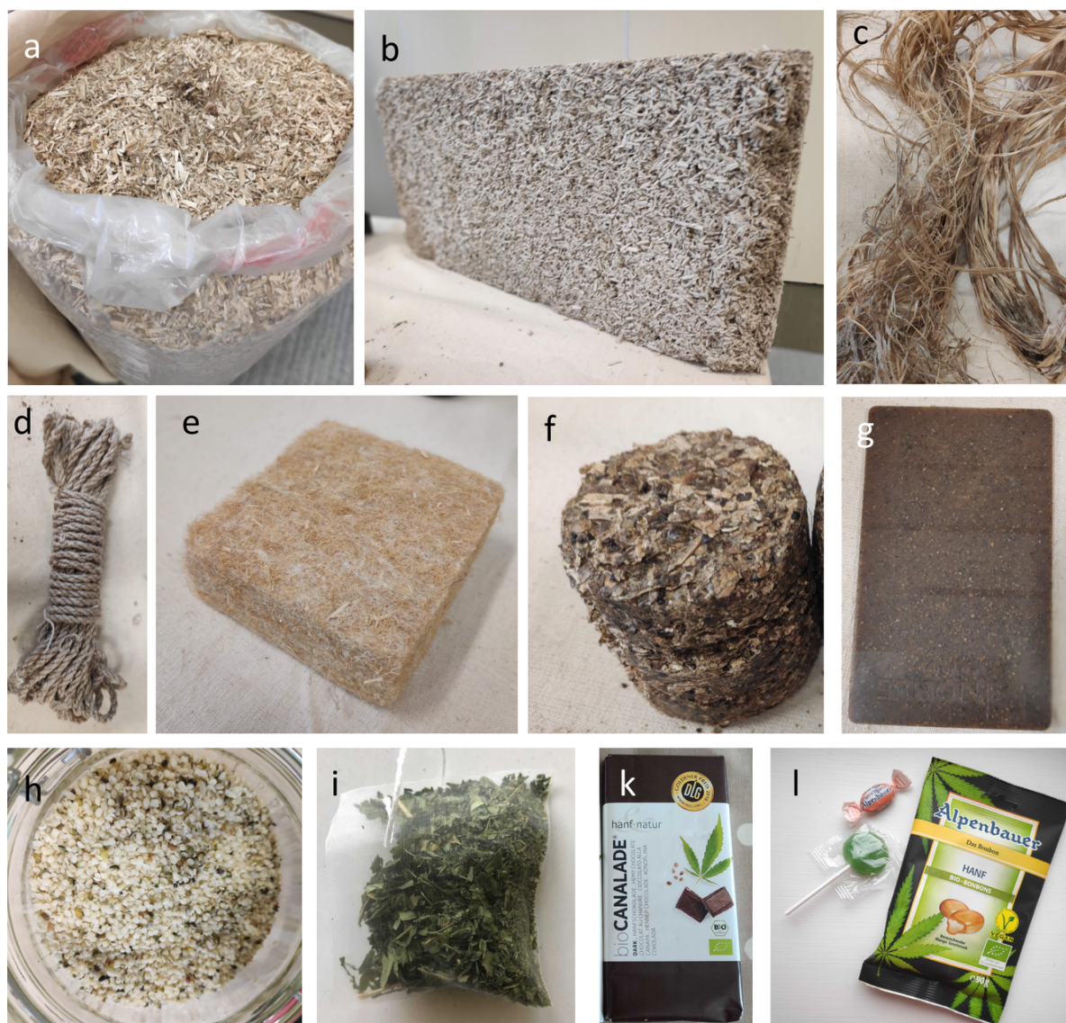
Figure 9: Products made from hemp. Non-THC Cannabis (hemp) can be processed into a multitude of different products. Hemp husk of fibre varieties (a) can be processed into hempcrete (b), while hemp fibre (c) can be made into rope (d) or insulation material (e). Remains of the plant can be pressed into hemp pellets for heating (f). Composite hemp-plastic material for 3D printing (g) is more sustainable than regular printing plastic. Hemp seeds can be dehulled into hemp hearts for human consumption (h). A variety of hemp products like tea (i), as well as chocolate (k) and candy (l) are also available. (i) courtesy of Christine Schilling.
