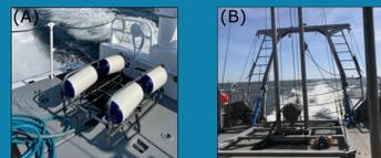
Figure 2. (A) Applied Acoustics boomer plate and catamaran; the boomer is towed with the blue HV cable attached and the hydrophone parallel from the vessel's stern. (B) The Rossfielder vibracore used during sediment core acquisition in 2019.
