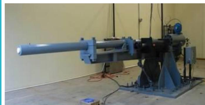
Utron (defunct) has developed a gas gun, it has much lower propellant costs than a conventional gun. The gentler acceleration reduces shell casing mass, and therefore improves payload fraction.
