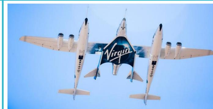
Virgin Galactic use the White Knight Two aircraft from Scaled Composites to carry SpaceShipTwo to its launch altitude. Similar two-stage launch technologies could be used to overcome the challenges of developing an aircraft optimised for both ascent and high-altitude cruise.
