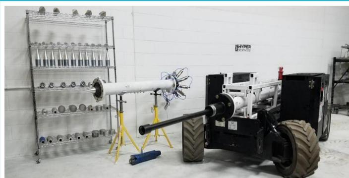
*Hypersciences use ram accelerator technology to drill rock. This mining cannon uses inexpensive propellant and experiences low barrel wear, despite having a high rate of fire. Their technology is also being developed for space launches.*
