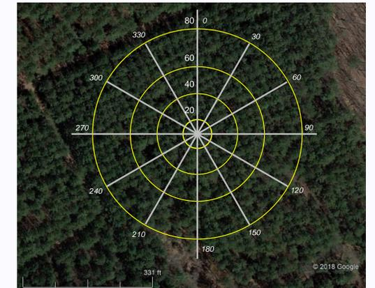
Data acquisition design options, showing concentric paths for orbit flights (including changes in camera pitch) and configuration for data collection including multiple azimuth angles.
