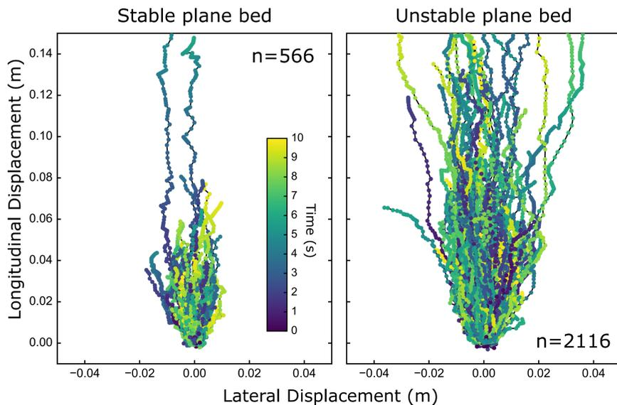
Visualization of tracer particle paths. Each plot shows all paths recorded over two ten second intervals (20 seconds total time represented for each condition).
