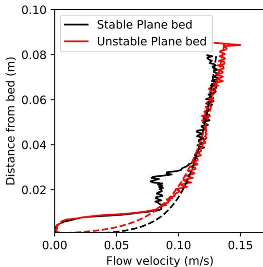
Ensemble average flow velocity profiles recorded using moving ADV.
